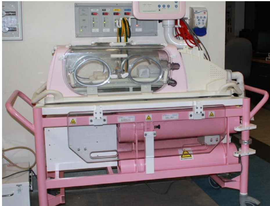
The BCCH MRI Research Facility MRI compatible incubator for neonatal scanning
