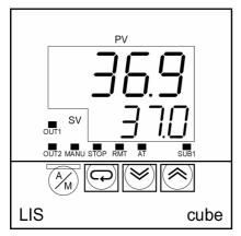
in the red main display. The smaller green digits below display the set temperature. The temperature control operates in real time and there is no need to confirm the set values by pressing an enter key.
